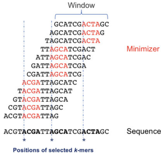
Fig. 1 A minimizers scheme. Given a sequence, in each window of length L = 12 , a minimizer of length k = 4 is selected (red). Consecutive windows are likely to select the same minimizer, and the selected positions constitute a sampling of the original sequence (blue asterisks)
